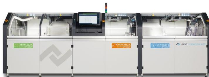
With its revolutionary flexibility, the soldering pots are able to move freely in x-, y- and z-direction. Each soldering pot is completely independent and has no y- or x-dependencies to the other one. An anti-collision software ensures the free movement of the servo-driven axis system of the soldering pots.
