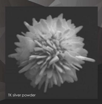
Introducing the **TK Paste**, a conductive adhesive developed using TK silver powder, the world's first thorny silver powder particles. TK Paste maximizes the advantages of TK silver powder by
